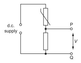
Which graph shows the variation with Celsius temperature  $\theta$  of potential difference V between points P and Q?
